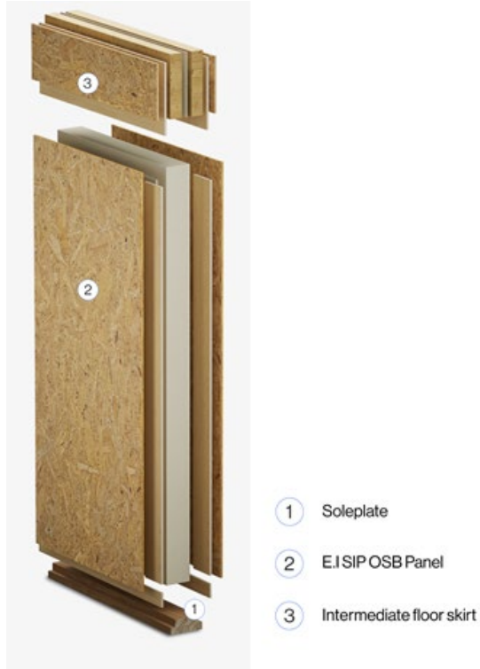
Diagram 1 - Panel, ring beam, baseplate and soleplate exploded detail
